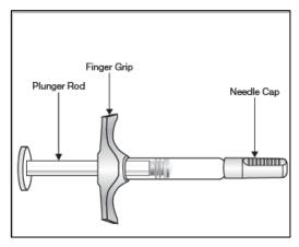
Figure A: HYRIMOZ prefilled syringe.
