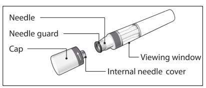
Figure A: HYRIMOZ Sensoready Pen parts
